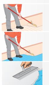
The surface of the VarioComp corresponds to the ÖNORM DIN 18202 (table 3, line 3), limits for levelness deviations (see also chapter 5).
