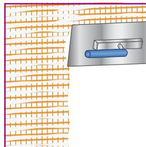
Apply finish coat plaster according to manufacturer's instructions and insert plaster lattice<sup>1</sup> close to the surface.
