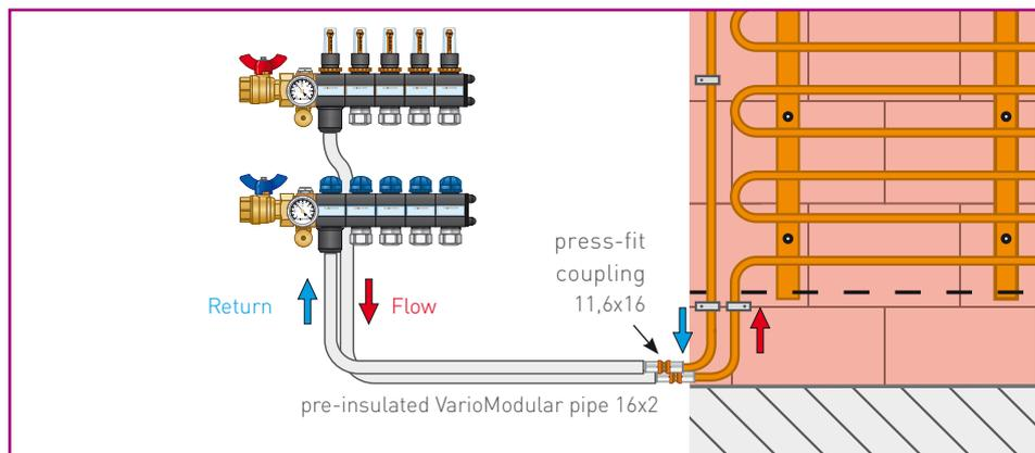
▲ Variant with pre-insulated VarioModular pipe 16x2 with press-fit coupling connection 11.6x16
