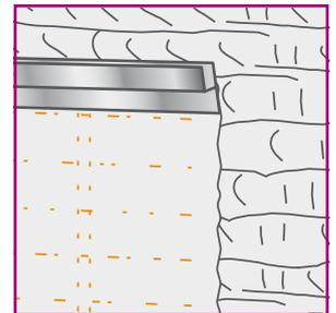
Skim down the first coat of plaster to the level of the VarioRail above the top of the pipe!
