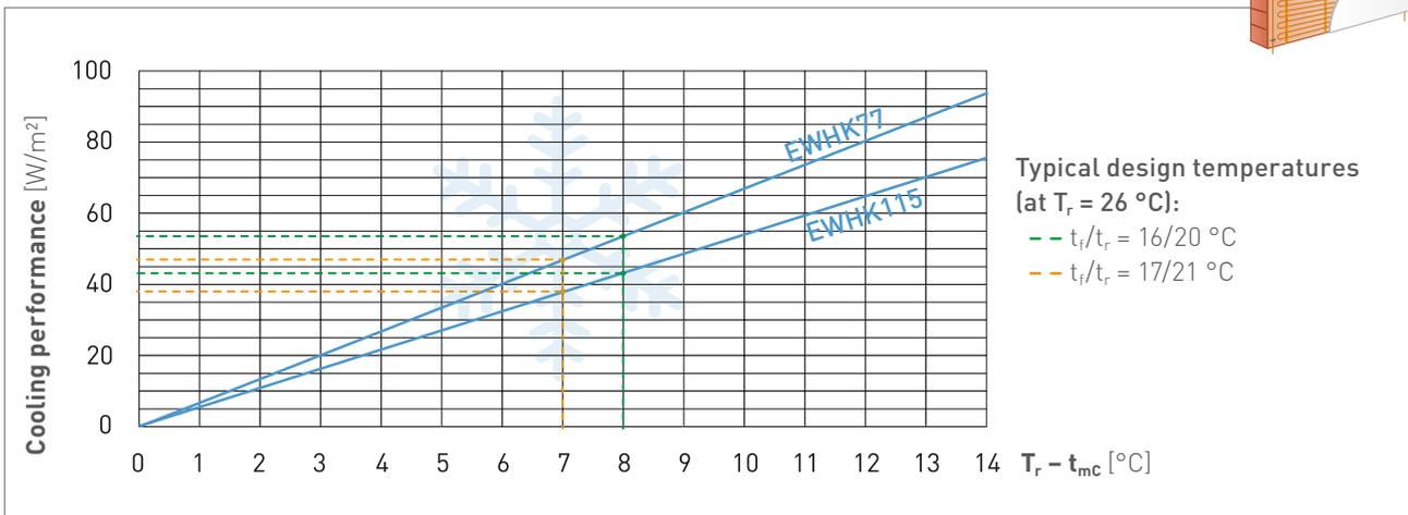
$$t_{mc} = \text{Mean cooling water temperature} = \frac{t_i + t_r}{2} \text{ [°C]}$$
