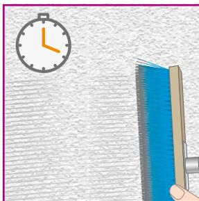
Allow EcoHeatingPlaster to set (6–9 hours) and roughen the surface slightly. **Do not damage the VarioProFile pipe!**
