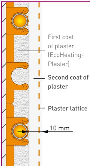
The **second coat of plaster is applied on site according to the manufacturer's instructions** on the first coat of plaster.
