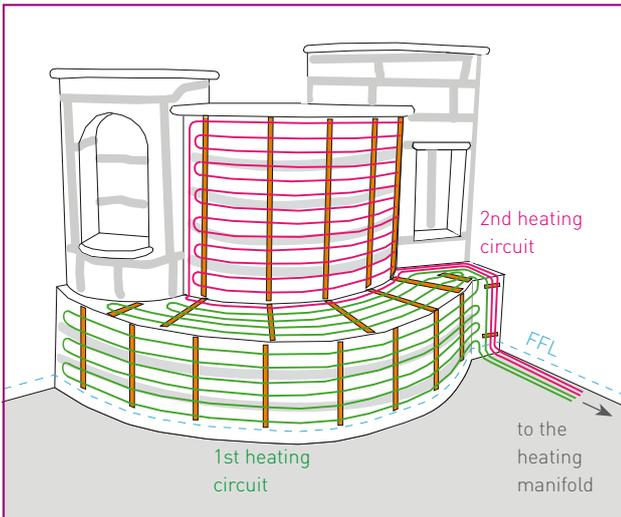
▲ Install the VarioProFile pipe 11.6x1.5
