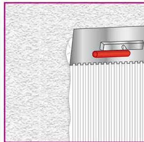
Apply skim coat according to manufacturer's instructions and the plaster lattice<sup>1</sup> ...
