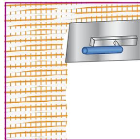
... work in and cover all sides with levelling compound.
