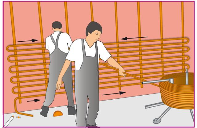
Maximum 11.6 mm pipe length per heating/cooling circuit
