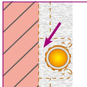
First coat of plaster also behind the VarioProFile pipe!
