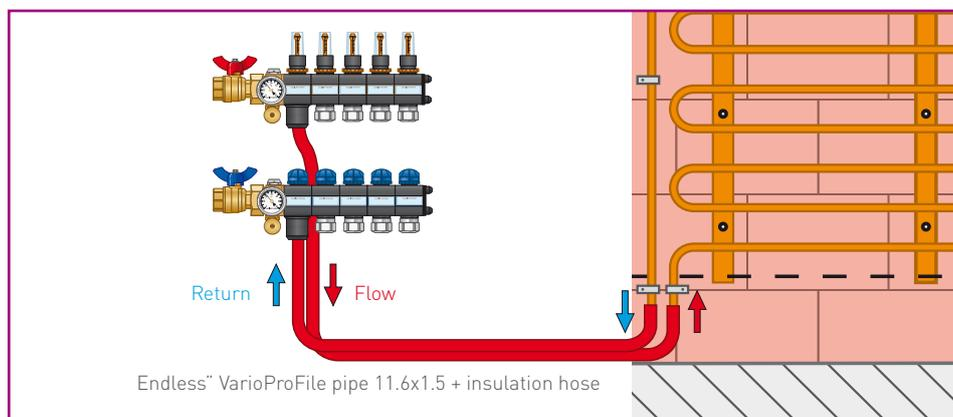
▲ Variant with Insulation hose 4 mm: "Endless" VarioProFile pipe 11.6x1.5
