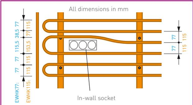
▲ For installations (sockets, windows, etc.), a smaller/larger section-wise spacing is permissible.
