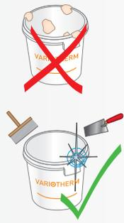
In order to prevent shortening of the pot life, empty the bucket completely after every mixing process with a trowel and clean it with a paint brush.
