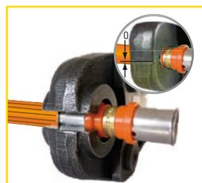
▲ Pressing. The press-fitting jaw must close fully.
