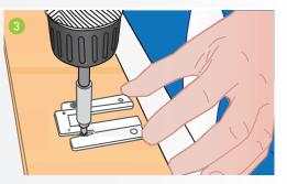
Screw the mounting base onto the upper cladding.
