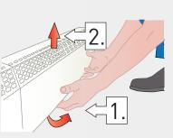
To remove the cladding, first pull it out at the bottom and lift it out upwards.
