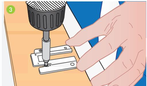
3 Screw the mounting base onto the upper cladding.
