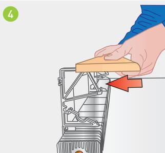
4 The upper cladding can now be pushed into place.
